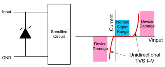
Figure 2. Application of a Unidirectional TVS Device
