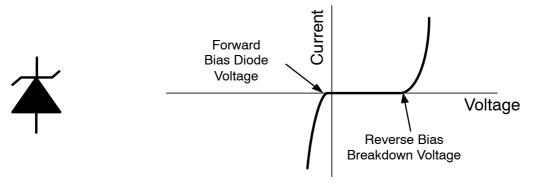
Figure 1. Unidirectional TVS Protection Properties
