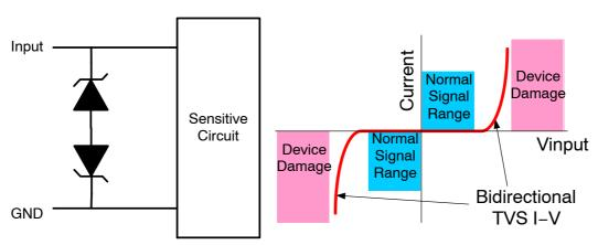
Figure 4. Application of a Bidirectional TVS Device
